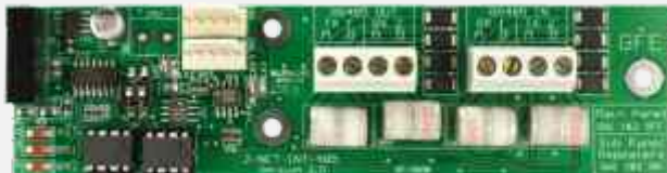
J-NET-INT-485 JUNO NET INTERFACE FOR RS485 COMMUNICATION
