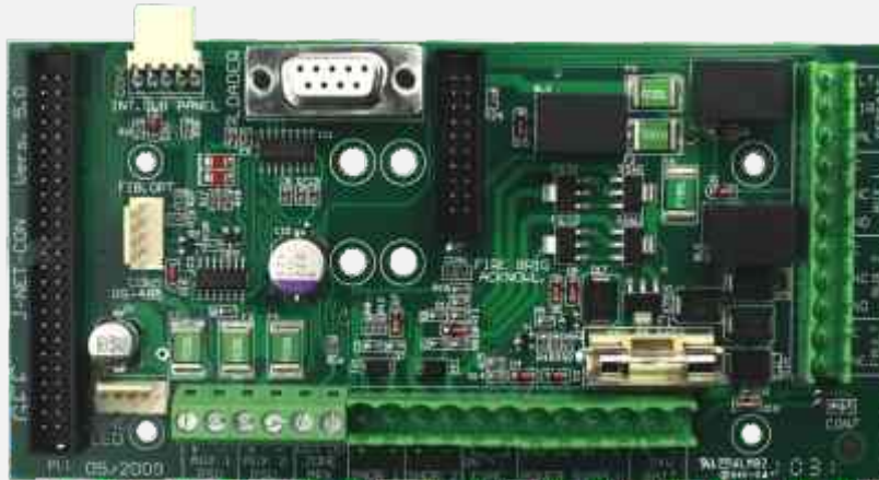
J-NET-CON JUNO-NET-CONNECTOR BOARD
